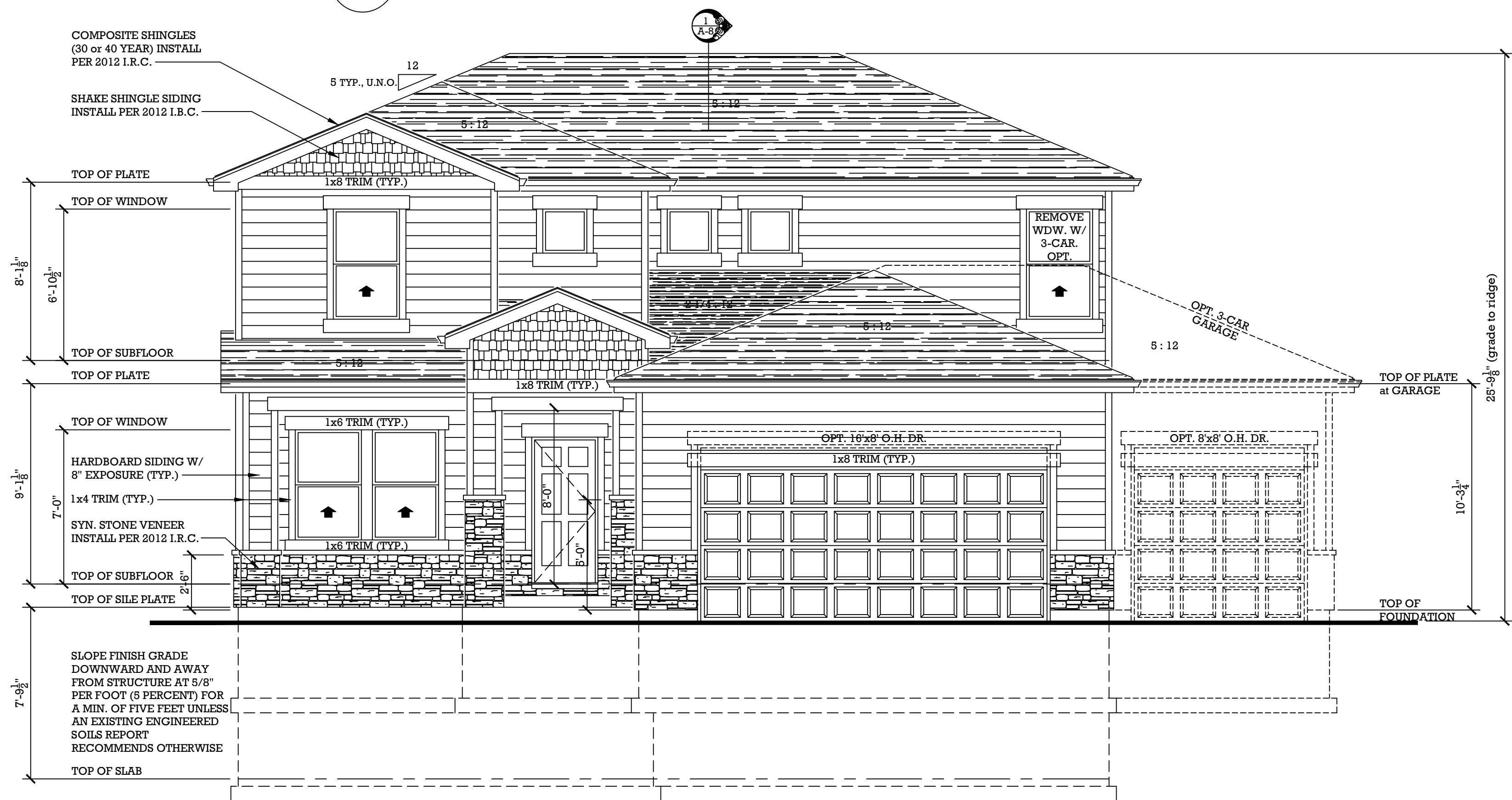
1 FRONT ELEVATION SCALE: 1/4"=1'-0"
