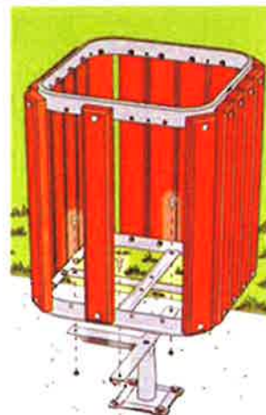
Model M3/G, M5/G, or M7/G: Surface Pedestal Mount for elevated installation of TRH-32s and TRH-32s, TRH-20s, or TRH-15s, respectively. A 2 3/8" O.D. steel pipe base, welded to structural steel angle cross arms, bolts to the base ring and is then bolted to the concrete surface. Hasp galvanized finish (denoted by /G in model numbers; for painted black enamel finish change /G to /B)
